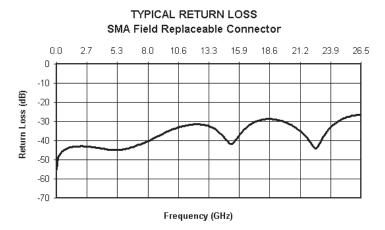
Although Johnson Components<sup>™</sup> does not publish a VSWR specification for field replaceable connectors, typical connector VSWR can be expected to be less than 1.1 + .01f (f in GHz). A VSWR specification is not stated because an industry standard method for testing field replaceable connectors does not exist. The actual performance of the connector is dependent upon the application for the following reasons:
