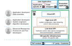
hardware platform enables you to extract depth data from the camera on the processor and operating system of your choice. Windows and Linux support are built into the SDK as well as sample code and wrappers for various languages including Python, C/C++ and MATLAB. The SDK also integrates with 3rd party technologies like OpenCV and RoS.
